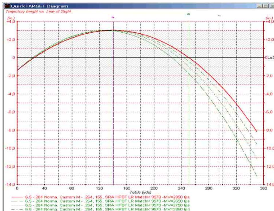
Picture 48: Comparing four trajectories, optimum zero ranges
