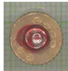
7,65 Parabellum, 3055 bar, 44300 psi No sign of high pressure.
