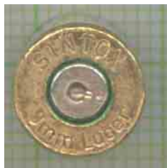
9 mm Luger, 3055 bar, 44300 psi Primer flattened, gap tightened, no further sign of high pressure
